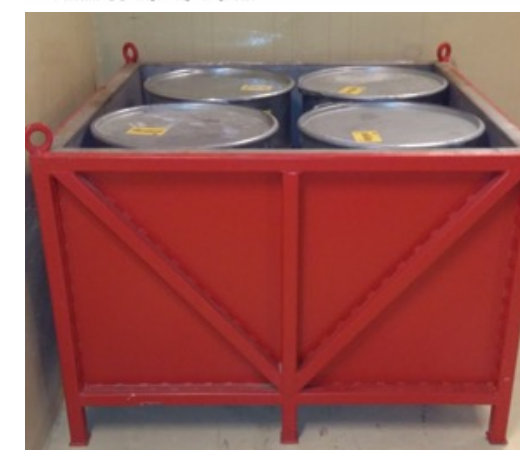
Barrels containing solidified sludge loaded in a shielded pallet.
